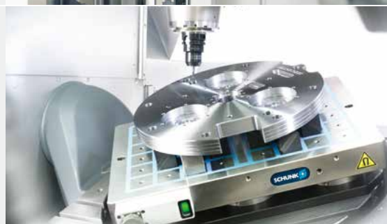
Magnetic clamping technology
